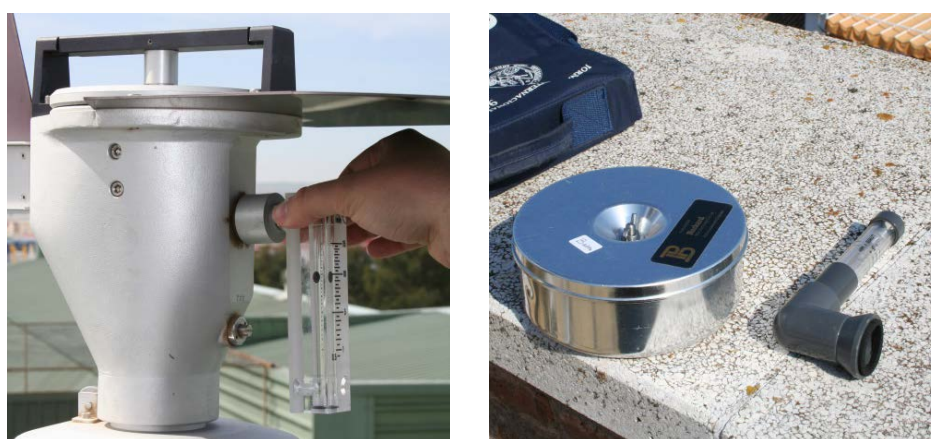
Figure 6.5 Flowmeters applied in the calibration of the spore traps. Two of the applied flowmeters in Córdoba, a Lanzoni (left) applied at the operational monitoring station and a Burkard Manufacturing (right) applied in a campaign on olive pollen monitoring.
