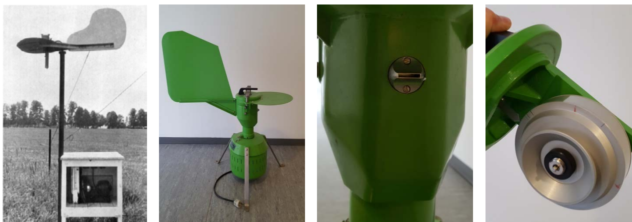
Figure 6.1 The original Hirst spore trap (Hirst, 1952) (far left), and a Hirst type spore trap from Burkard; orifice and drum (center and right), currently applied for research purposes at Aarhus University.
