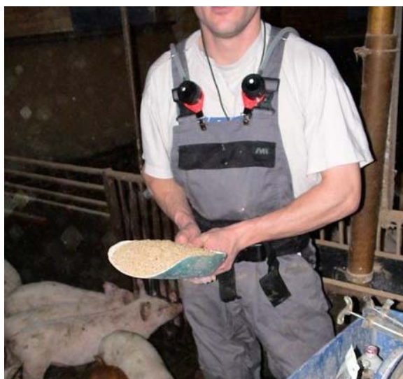
Figure 4 A farmer with the two GSP samplers clipped near his breathing zone while hand feeding weaners.
