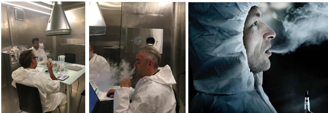
Figure 3.8. E-cigarette users vaping in the adjacent chamber. The aerosol was transported to the exposure chamber by a funnel in the ceiling connected to a pipe leading into the exposure chamber. Pictures: Private.
