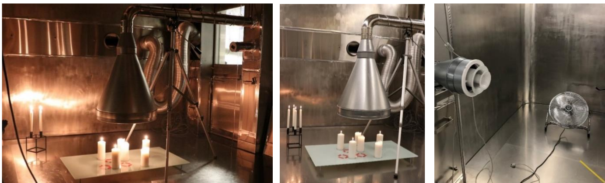
Figure 3.9. Pictures to the left showing the candle exposure set-up (pictures show the initial burning phase, which was not included in the trial). Picture to the right: Polluted air dispersed into the exposure chamber through an inlet and mixed with existing air by a fan. Pictures: Private.
